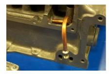
Step 4 Work the curved connection tube into the main oil supply hole until the tube can be rotated up to fit behind the exhaust valve boss. (Because some mian oil supplies vary slightly in size this might take a bit of work to get installed) At this point, the threaded brass opening of the curved oil connection tube should be pointing out of the engine. (second picture)
